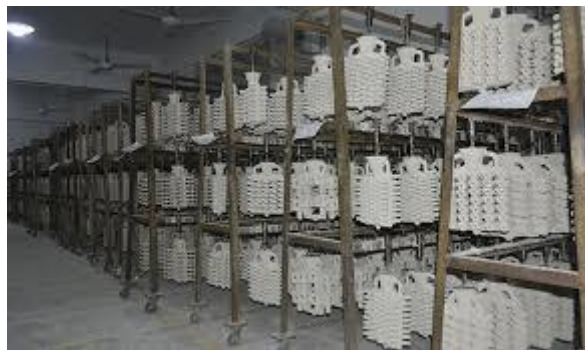
Gambar 2. 9 Proses pengeringan Dipping
