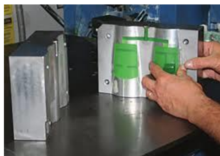
Gambar 2. 5 Proses Wax Injection
