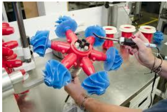
Gambar 2. 7 Proses Wax Assembly
