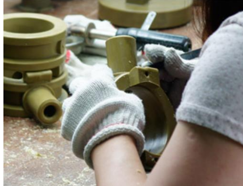
Gambar 2. 6 Proses Fixing Wax
