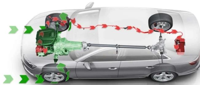
**Gambar 2. 9 Aliran Energi Pada Saat Proses *Regenerative Braking***
