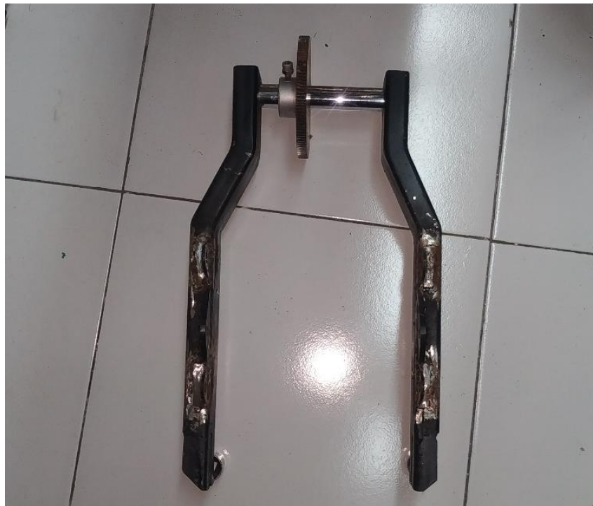
Gambar 4.1 Hasil Redesign lebar Swing Arm
