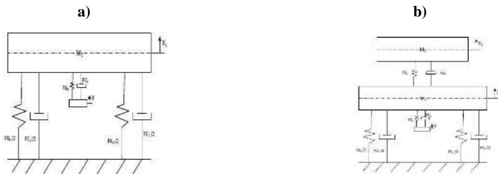
Gambar 2. 10 (a) Main system dynamic model and (b) Main system dynamic model with addition of CPVA (Zulfianti, 2019)
