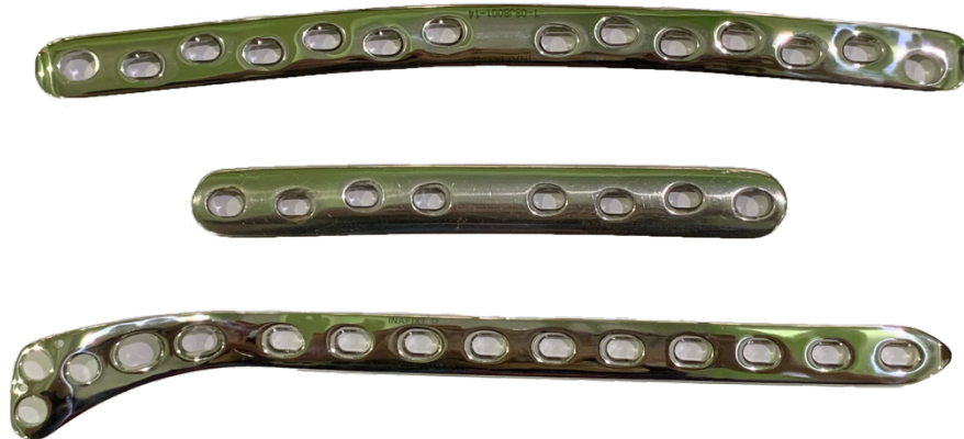
Gambar 2. 1.Implan Tulang Stainless Steel 316L (PT. Pelopor Implantindo)
