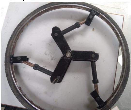
Gambar 2.15 Fabricated in-wheel suspension (Gowri et al, 2020)
