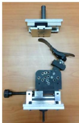
Gambar 2.10 Pengujian *Ankle-Foot Prosthetic* Berdasarkan Standar KSP 8403 (Song et al., 2019)
