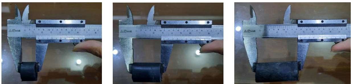
Gambar 3. 21 Rubber with Variation Length (a) 15 mm, (b) 30 mm, and (c) 45 mm
