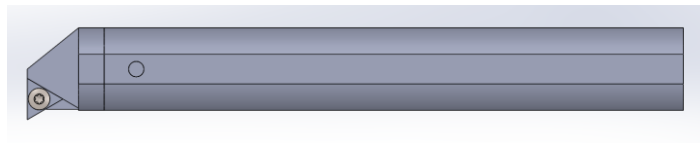
Gambar 3. 4 Customized Boring Bar Top View
