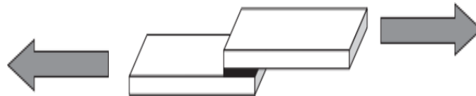
Gambar 2.3 Sambungan single lap (Goss, 2010)
