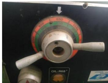
**Gambar 3.27** Spindle Rotation Variations on a Lathe Machine
