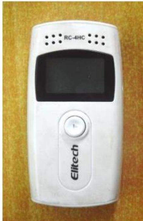
**Gambar 3.6** RH Meter Elitech Tipe RC-4HC
