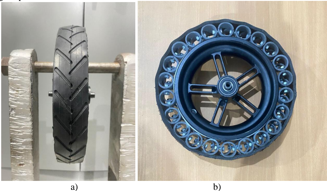
Gambar 4.5 a) Ban airless tampak depan b) Ban airless tampak samping
