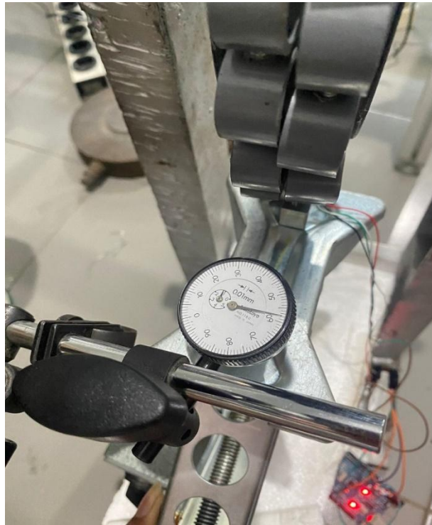
Gambar 4.8 Uji Deformasi Spoke
