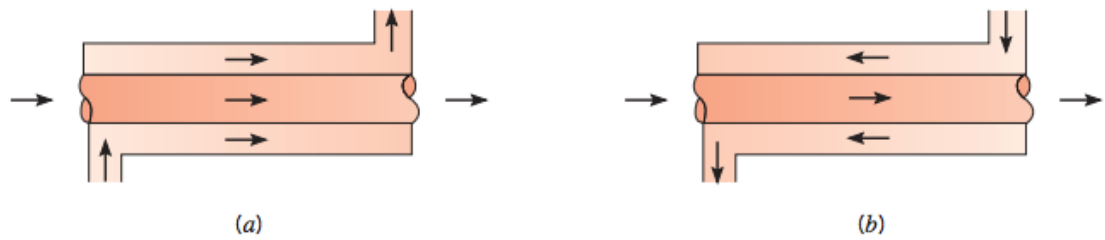
Gambar 2.10. Concentric tube heat exchanger a) paralel flow b) crossflow (Incropera, Bergman, & Lavine, 2011)
