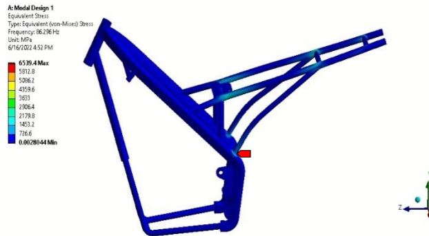
Gambar 4.6. Equivalent stress Desain 1 Mode Shapes 1
