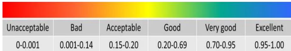
Gambar 3. 16 Orthogonal Quality Mesh Spectrum
