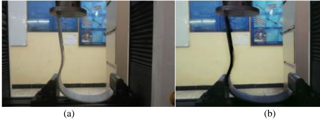
Gambar 2. 44 Uji Defleksi pada Spesimen; (a) Glass Fiber , (b) Carbon Fiber (Abood & Habeeb, 2019)
