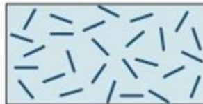
Gambar 2. 13 Randomly Oriented Discontinuous Fiber (Gibson, 1994)
