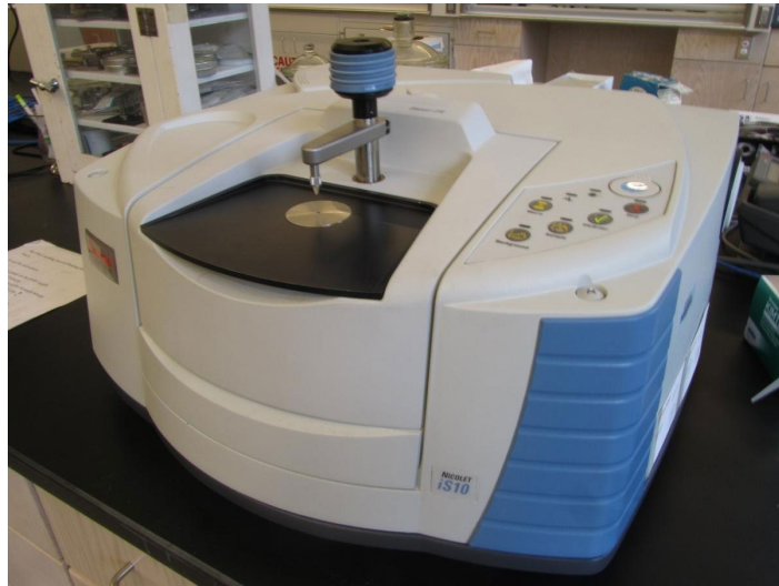
Gambar 3. 9Mesin FTIR Nicolet iS10 Spectrometer (Stone, n.d.).
