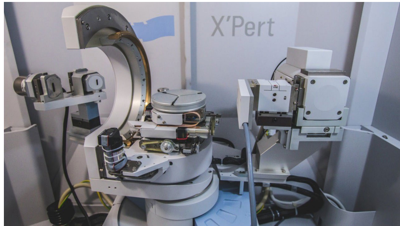
Gambar 3. 8 Mesin X-Ray Diffraction X'pert PRO PANALytical (University of California, n.d.).
