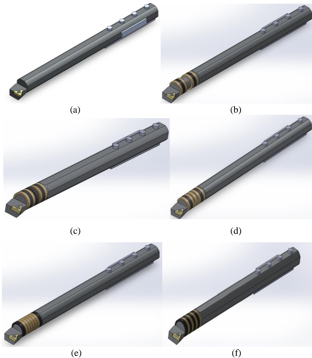
Gambar 3. 26 Customized Geometry Boring Bar with 6 Position Variations of DVA Rubber
