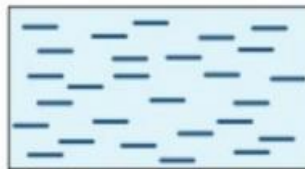
Gambar 2.12 Aligned discontinuous fiber (Gibson, 1994)
