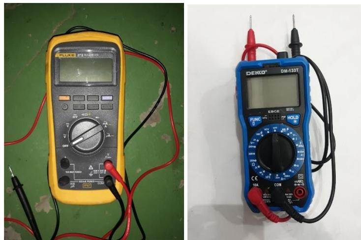
**Gambar 3. 20** *Multimeter*
