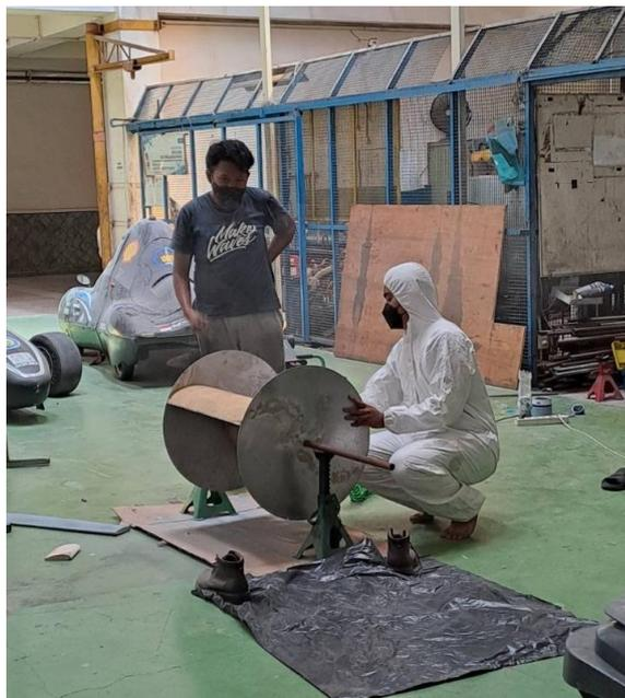
**Gambar C. 4** Proses Pengecatan Turbin Savonius
