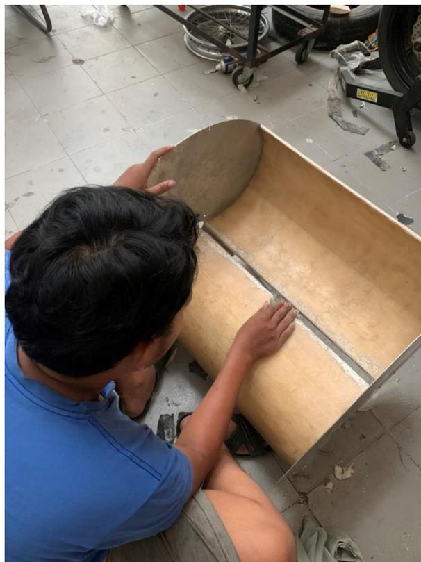
**Gambar C. 2** Proses Pengamplasan Turbin Savonius
