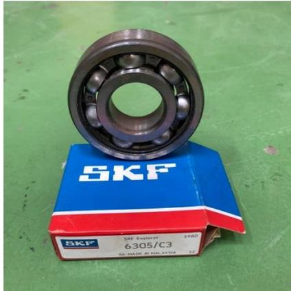
**Gambar 3. 14** *Ball Bearing SKF 6305/C3*
