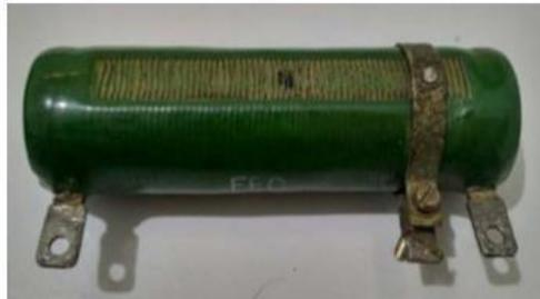
**Gambar 3.28** *Resistor* tipe wirewound
