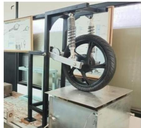
**Gambar 2.10** Mekanisme *Regenerative swing arm* (Suryana,2022)
