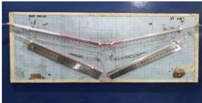
Gambar 3. 9 *Inclined Manometer (Manometer V)*
