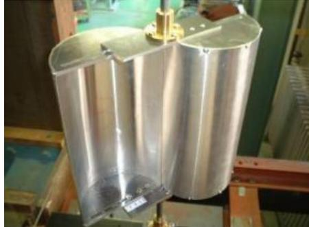
**Gambar 2.5** *Vertical Axis Wind Turbine* tipe Savonius (Vanessa, 2016)
