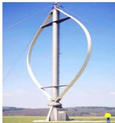
**Gambar 2.4** *Vertical Axis Wind Turbine tipe Darrieus eggbeater (Aboufares, 2015)*
