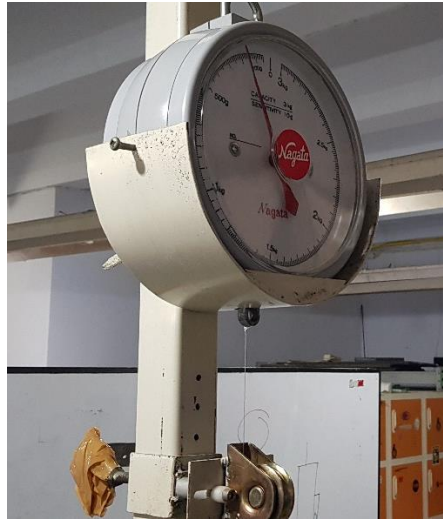
Gambar 3. 14 Neraca Pegas NAGATA C-5
