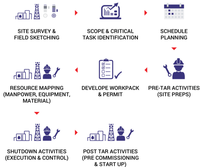
Gambar 2.1 Standar Proses Turnaround Maintenance ( www.mesitechmitra.co.id )
