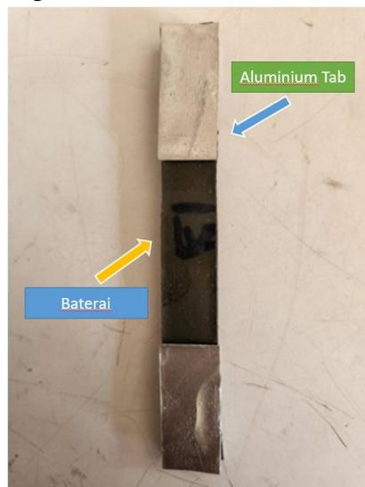
**Gambar 4.15** Spesimen *Tensile test* ASTM D3039
