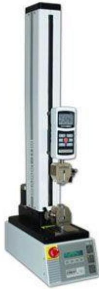
**Gambar 3.4** Universal Testing Machine Mark-10 ESM301L (Lab Metalurgi DTM-ITS)
