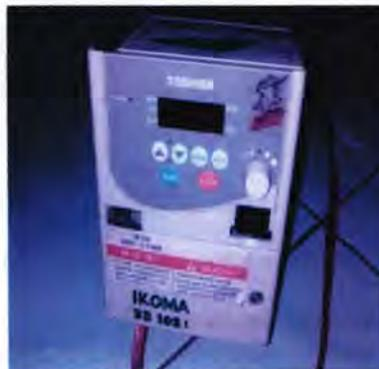
**Gambar 3.10** *Inverter* Toshiba VF-S9
