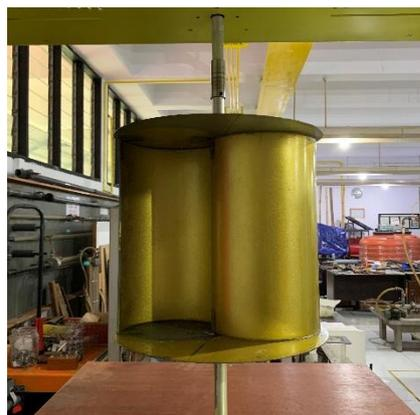
**Gambar 3.6** Turbin Savonius
