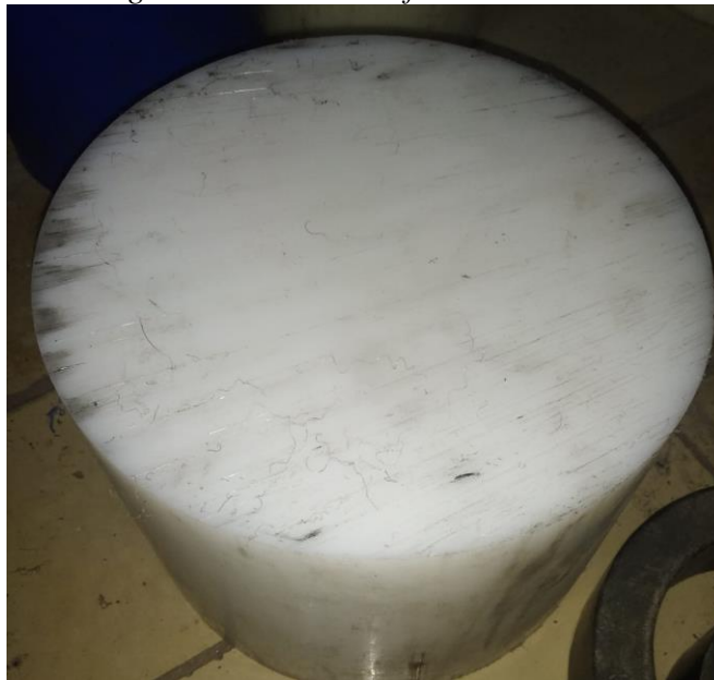
Gambar 4. 40 Raw Material Polyethylene Diameter 250 mm Tebal 100 mm
