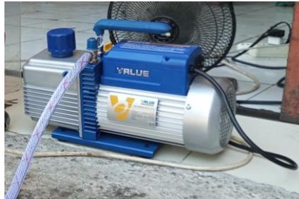
*Gambar 4. 5 Pompa Vakum*
