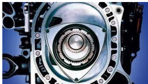
Gambar 2. 3 mesin rotary ( https://otodriver.com/berita/2019/mesin-rotary-mazda-bakal-digunakan-kembali-mesbjdfaali )
