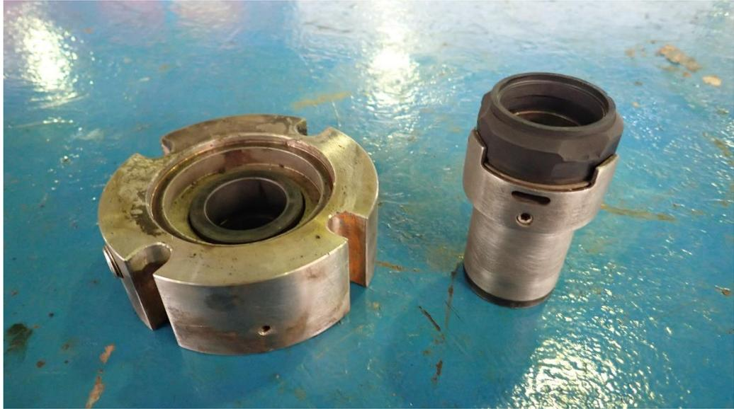
*Basic Mechanical Seal Pompa FC-P-754B*
