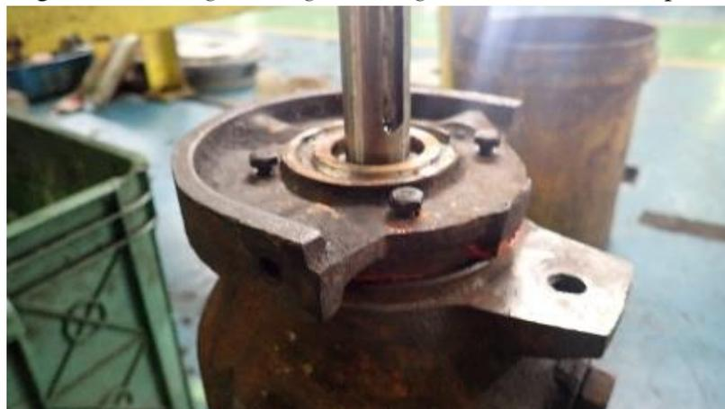
**Gambar 4. 33** Memasang *Cover Bearing Housing* beserta *Gasket*
