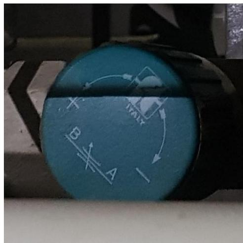
**Gambar 4.27** *Adjustable Flow Rate Valve*
