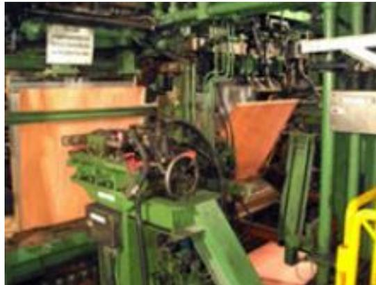
**Gambar 2.17** *Cathode Washing and Stripping Machine* (CWSM)
