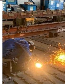
Proses Air Arc Gouging
