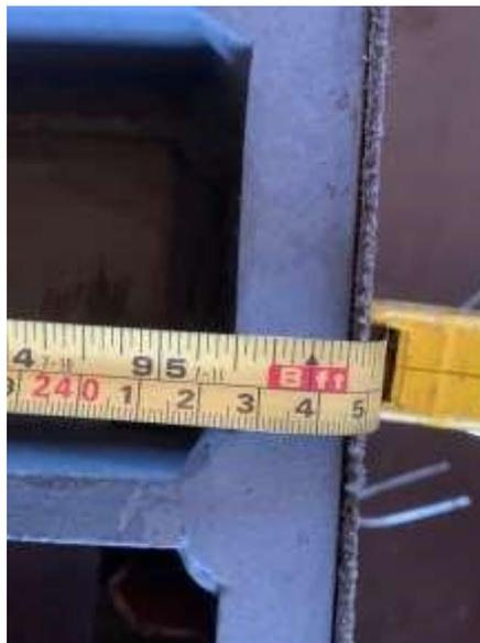
**Gambar 4. 49** Dimensi Sebelum PWHT (*Post Weld Heat Treatment*)
