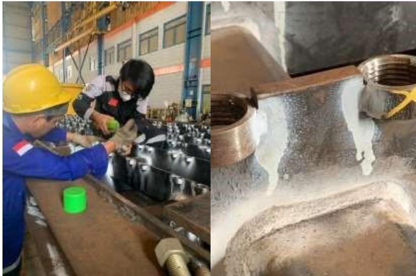
**Gambar 4. 36** Proses MPI (*Magnetic Particle Inspection*)
