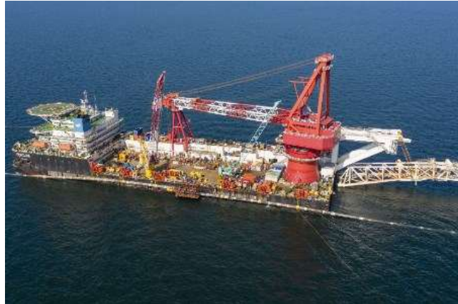
Gambar 2. 2 Tie-In Vessel (Knight, 2021)
