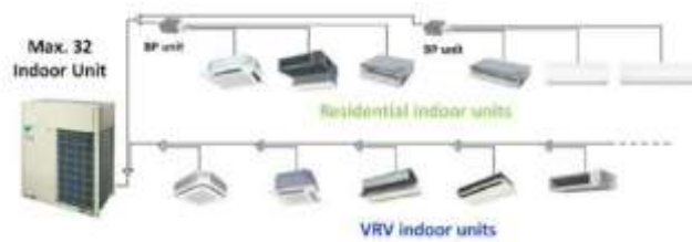
Gambar 2.17 Variable Refrigerant Volume / Variable Refrigerant Flow
