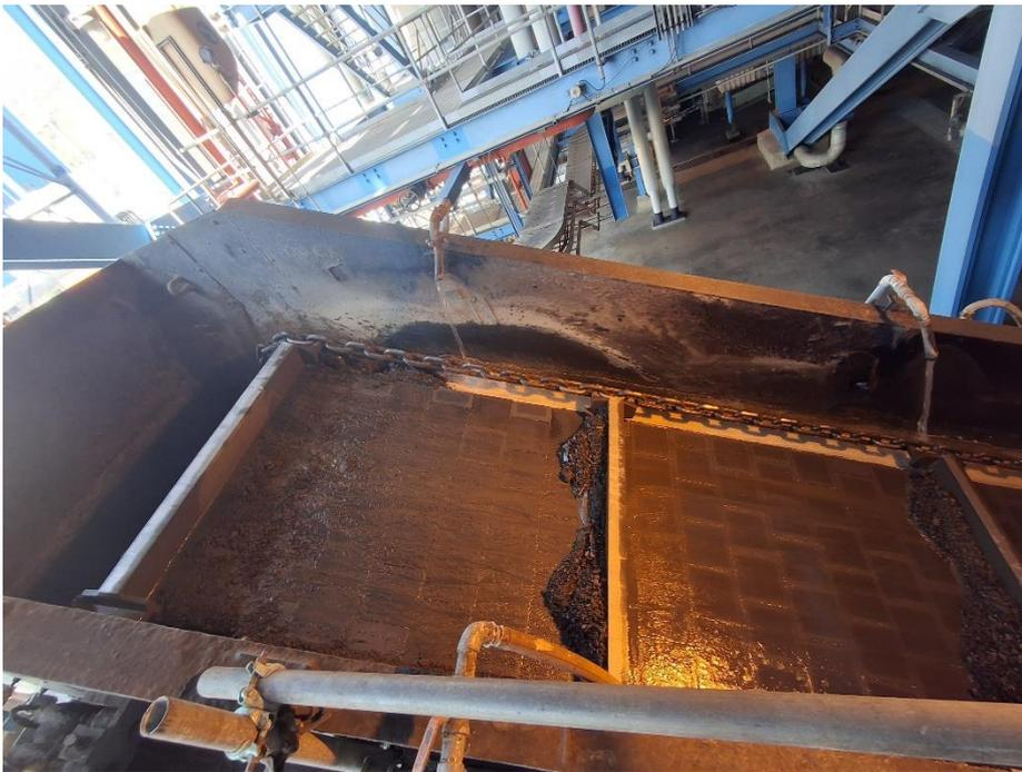
**Gambar 2. 22** *Submerged Scrapper Chain*
