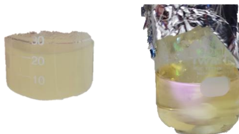
Figure 4.2 Visual testing of PAN/CsPbBr 3 (a) Regular condition (b) Under UV light
