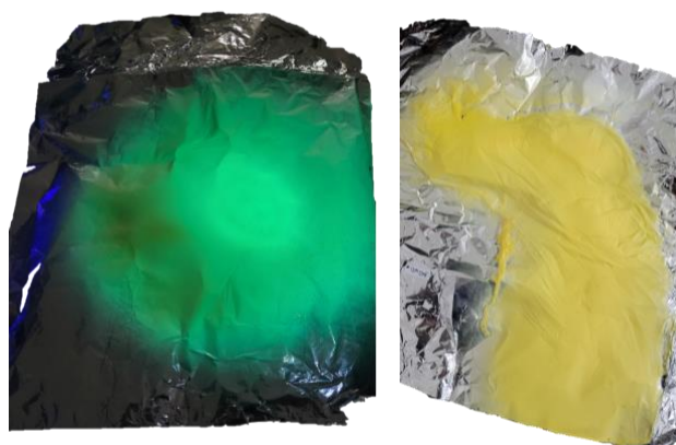
Figure 4.3 Visual testing of PAN/CsPbBr 3 nanofiber membrane under UV light condition in all three composition (a) 1:2 (b) 2:3 (c) 1:1.
