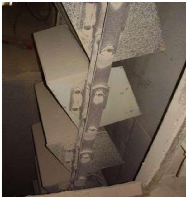
**Gambar 2.18** Drag Conveyor M-2205
