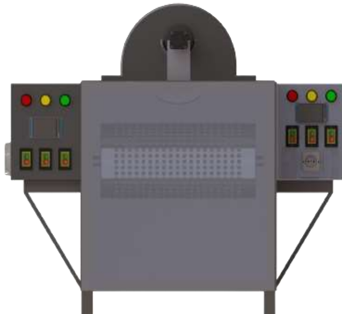
Gambar 3. 11 Tampilan Integrasi Chipper dan Dehydrator Tipe Rotary Cylinder
