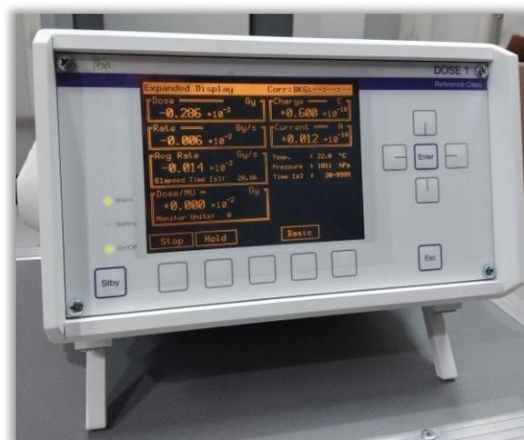
Gambar 3.4 Elektrometer IBA Dose 1
