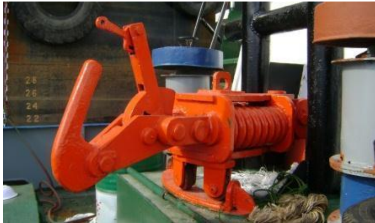
Gambar 2. 2 Towing Hook (Sumber: https://kisahyd.blogspot.com/2020/11/towing-and-lashing )
