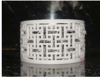
Gambar 3.14 Hasil 3D Printing Auxetic Tube
