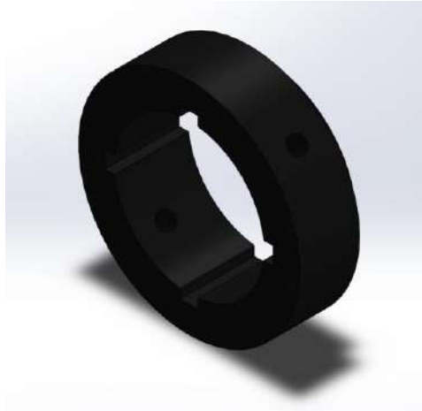
Gambar 4.7 Desain 3D Hub Screw
