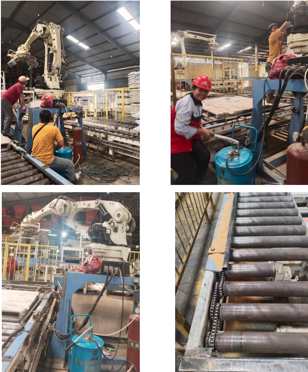
Gambar 3. 9 Maintenance Pergantian Pelumas / Grease
