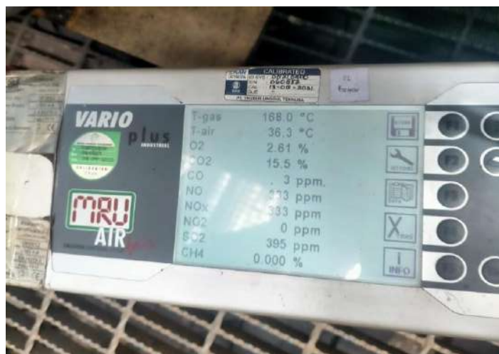
Gambar 4. 9 Alat Ukur MRU Vario Luxx Emission
