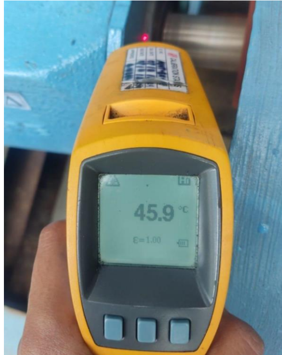
Gambar 4. 11 Alat pengecek temperature bearing ( Infrared Thermometer )
