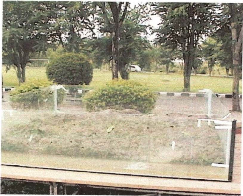
Gambar 3.2 Reaktor Rainfall simulator
