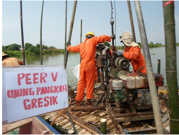
Figure 3.1 Process of sediment sampling (a) the barge (b) sediment sampling at Location 1 (c) sediment sampling at Location 5
