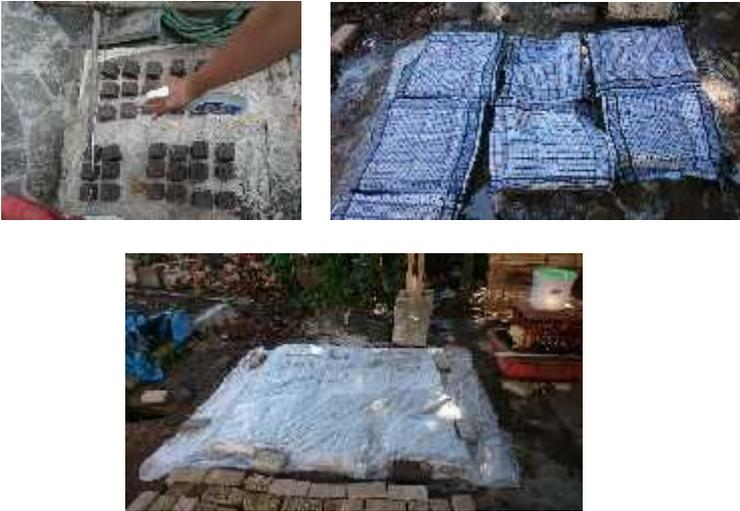
**Gambar 4.26** Proses perawatan / *curing paving* geopolimer.
