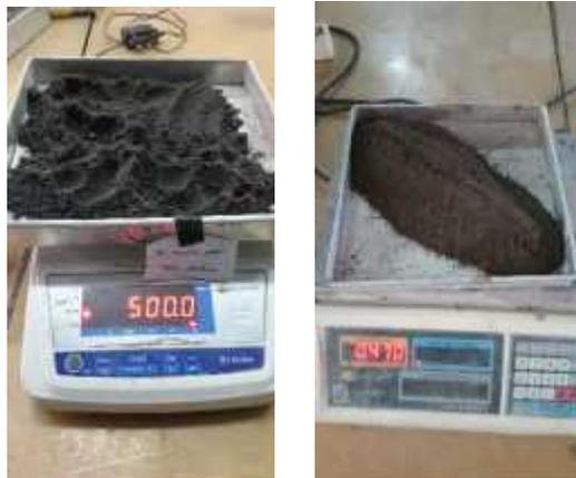
**Gambar 4.19** Proses Uji Air Resapan *Bottom Ash*
