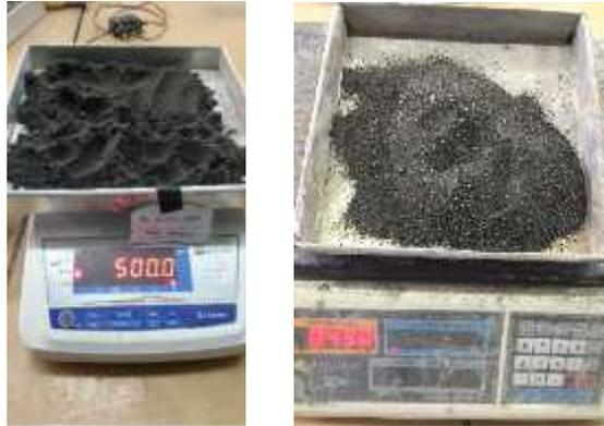
**Gambar 4.3** Proses Uji Air Resapan Pasir
