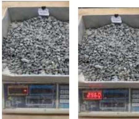
**Gambar 4.15** Proses Uji Air Resapan batu pecah
